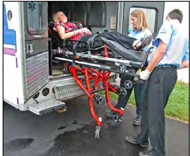
Figure 20 - After the Control-End Legs Unfold, Check the Indicator to Verify the Legs Have Locked
