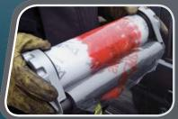
To start: The film must be sticky side up and over the leading roller. Only pull a small amount of film away from the roll, as shown.
