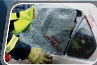
After breaking the glass, use a glove cover to remove glass in one piece.
