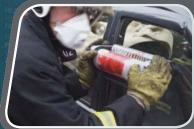
Application: Both rollers must stay in contact with the glass and in a level position; ensuring controlled application, reducing air bubbles and creases.
